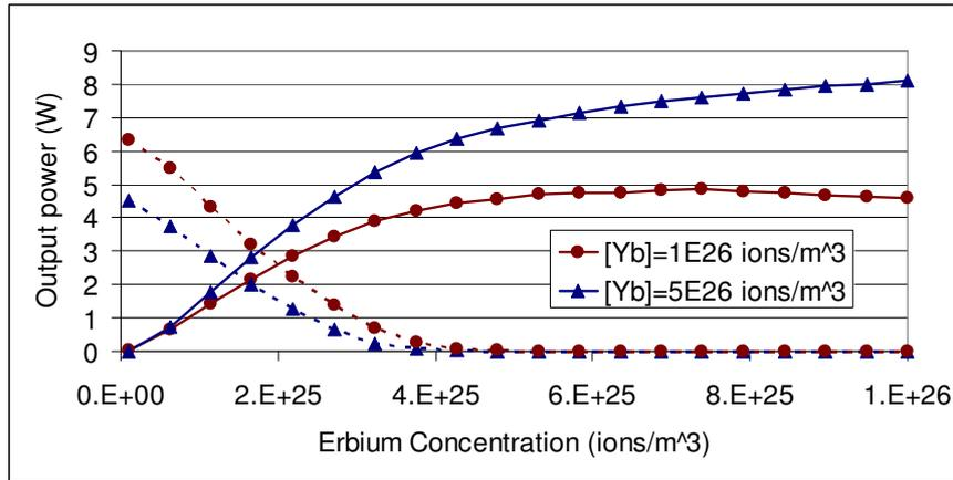
Figure 5. Output signal power (full line) and ASE at 1.0  $\mu\text{m}$  (dashed line) as a function of erbium and ytterbium concentration for an amplifier seeded with 5 mW at 1563 nm and pumped in counter-propagation with 25 W at 915 nm. Two different ytterbium concentrations are used: circle and triangle points represents ytterbium concentration of  $1 \times 10^{26}$  and  $5 \times 10^{26}$  ions/m<sup>3</sup> respectively.
