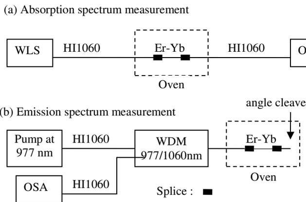
Figure 1. Setup to measure the relative variation of the absorption spectrum (a) and the relative variation of the emission spectrum (b) as a function of temperature.
