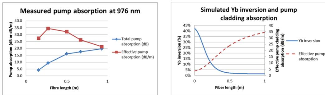
Fig. 2. Pump absorption of the 20/128 Yb fiber at 976 nm. (left) and simulated Yb inversion and pump absorption (right)
