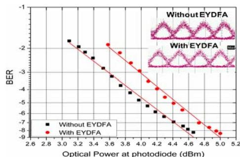
Fig. 3. Bit error ratio and eye diagrams (inset) at 40 Gb/s with and without the EYDFA in the communication link.
