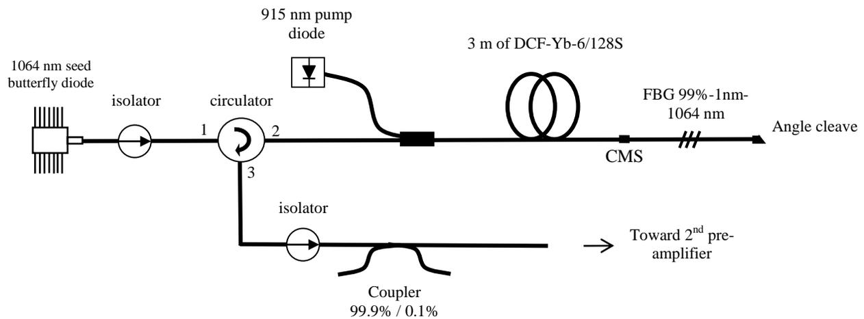
Figure 2. Detailed schematic of the first pre-amplifier used
