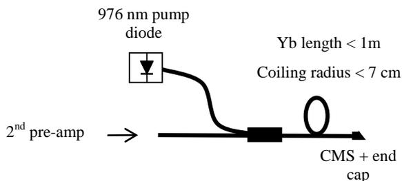
Figure 4. Detailed schematic of the power amplifier
