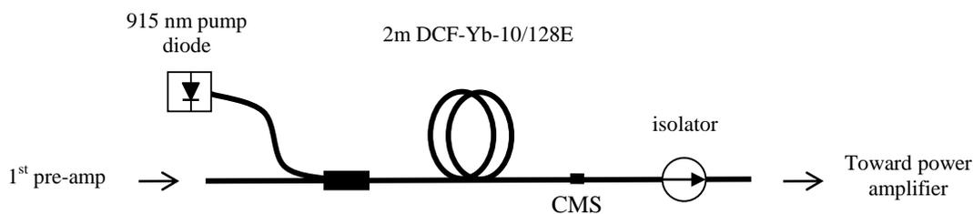
Figure 3. Detailed schematic of the second pre-amplifier
