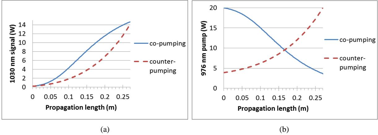
Figure 15. Simulation of the propagating power when pumping 0.27 m of DCF-Yb-20/128P-FA with 20W of pump power at 976 nm when injecting an input signal of 0.2 W at 1030 nm: evolution of (a) signal power and (b) pump power
