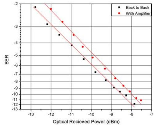
Fig. 4 Bit error ratio at 10 Gb/s with and without the EYDFA in the communication link.
