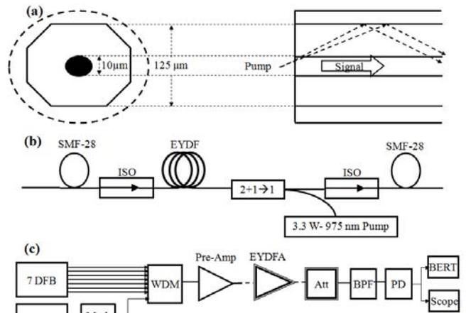
Fig. 1. Schematics of (a) the EYDF, (b) the EYDFA, and (c) the bit error ratio measurement setup. Mod: modulator, BPF: bandpass filter@1544 nm, Att: variable attenuator, PD: Photodiode, BERT: BER tester.
