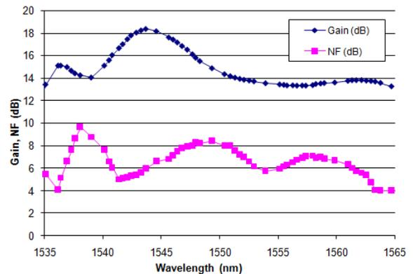
Fig. 3 Gain and noise-figure of the EYDFA taken alone.
