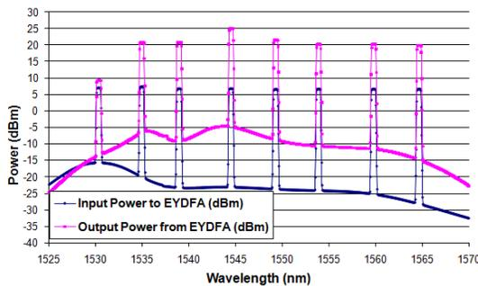
Fig. 2 Spectra before and after amplification of 7 channels spreading from 1535 nm to 1565 nm.
