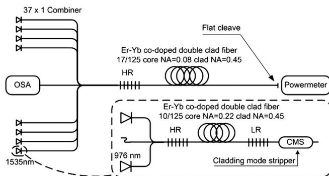
Fig. 1. High-power 1585 nm fiber laser configuration. Thirty-six fiber lasers emitting 11 W each at 1535 nm are used to pump an 18 m long Er–Yb codoped laser cavity. HR, high-reflectivity fiber Bragg grating; LR, low-reflectivity fiber Bragg grating; CMS, cladding mode stripper; OSA, optical spectrum analyzer.
