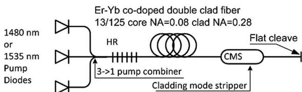
Fig. 4. Experimental setup used to compare pump wavelength efficiency. A silica cladding (NA = 0.28) Er–Yb codoped fiber laser cavity is pumped at either 1480 or 1535 nm.
